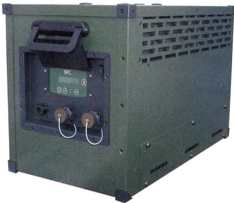
The FC 250 fuel-cell system has a nominal output of 250W, giving it a daily charging capacity of 6kW hours. It can power equipment on large military vehicles or do duty as a field generator. It has been designed especially for military applications including test scenarios in which data on new defence systems need to be collected and evaluated in the field. (Photo: SFC Energy)
